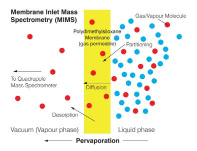
The Hiden HPR40 Membrane Inlet Mass Spectrometer (MIMS) is a compact bench-top gas analysis system for quantitative analysis and monitoring of dissolved/evolved gases.
